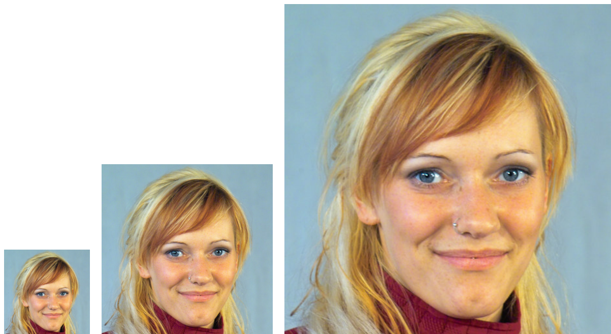
Figure A-2 – Resolution separation in geometric progression – Property of many image coding techniques.
